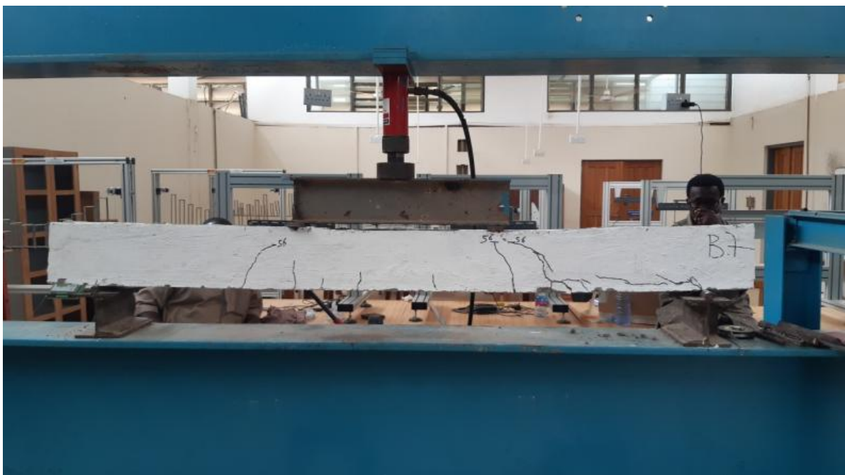
Fig. 15. Beam 7 failure mode
