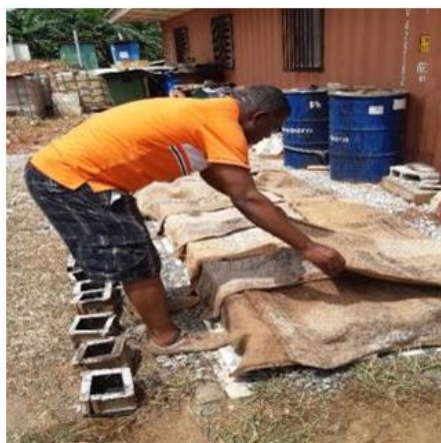
Fig. 3. Curing of specimens
