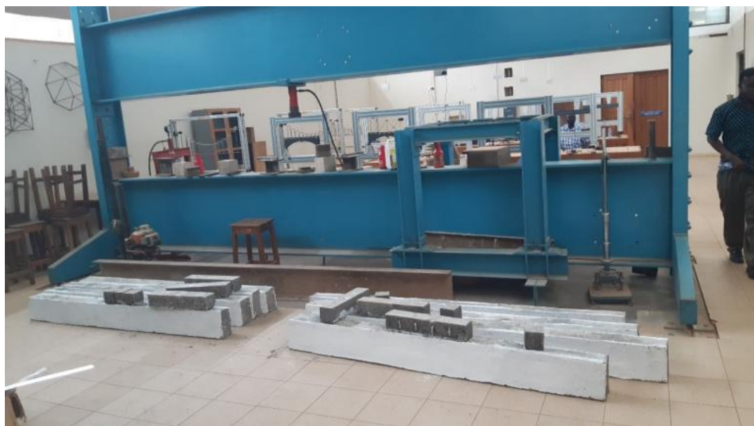
Fig. 6. Concrete beams ready for testing
