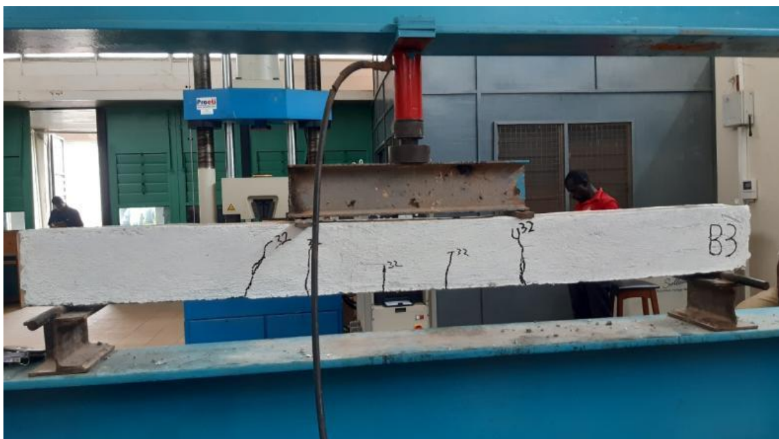
Fig. 11. Beam 3 failure mode
