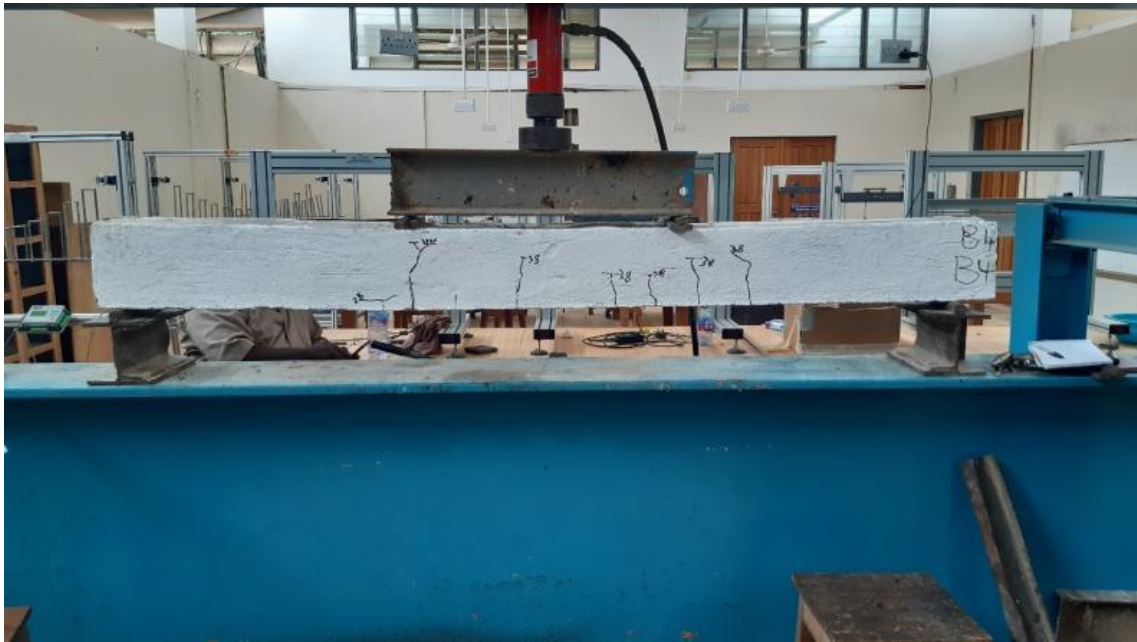
Fig. 12. Beam 4 failure mode
