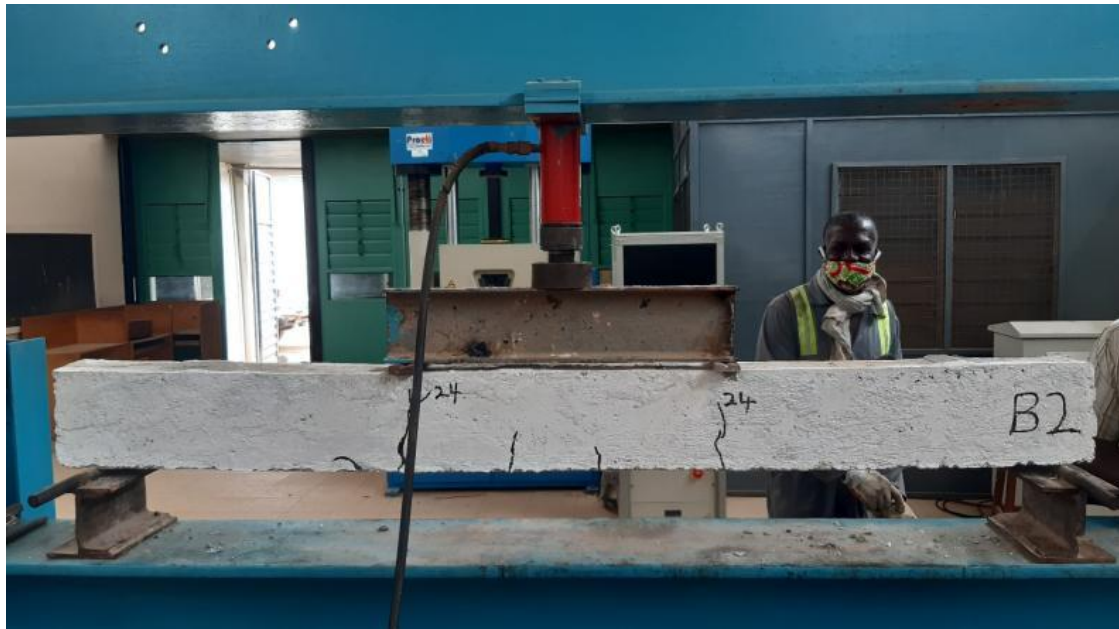
Fig. 10. Beam 2 at failure
