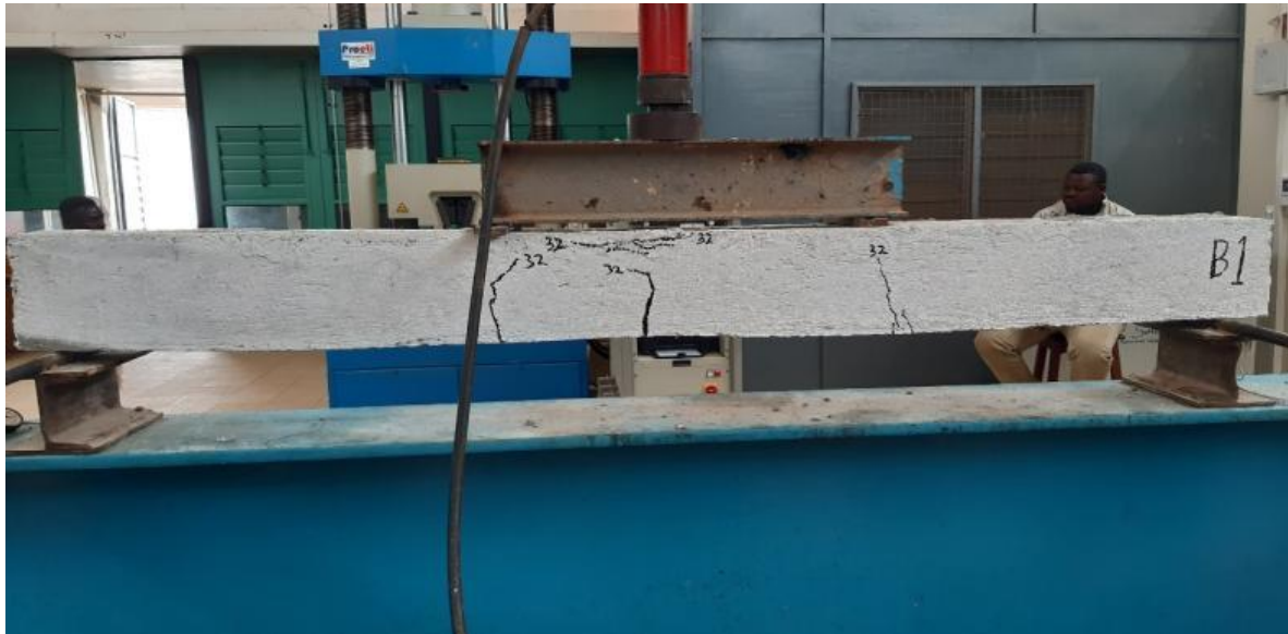
Fig. 9. Beam 1 at failure
