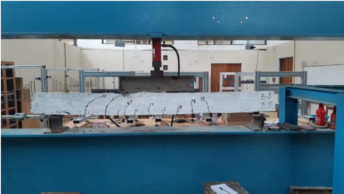
Fig. 16. Beam 8 failure mode
