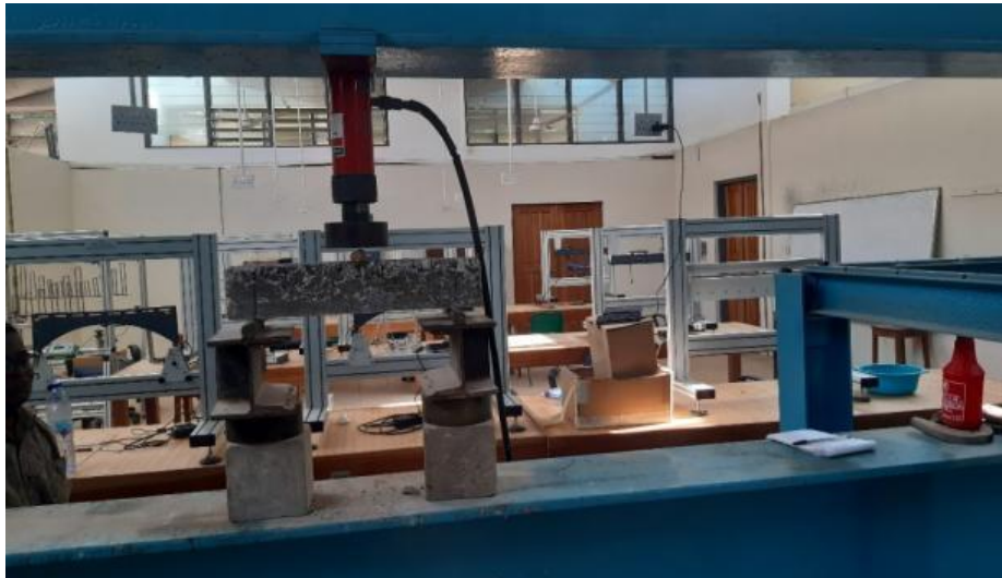
Fig. 5. Flexural test on concrete prism
