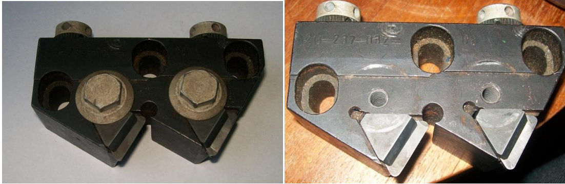
Fig. 7. Integrated cutting tool with two replaceable inserts
