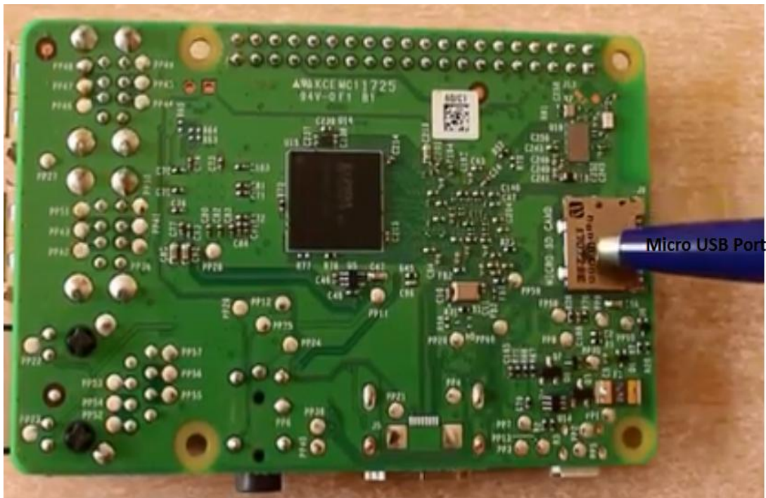
Fig. 3. Raspberry Pi single board back view features
