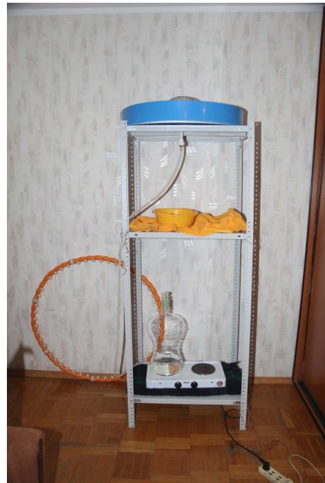
Fig.14. The rack with a tray, a glass bulb and electric stove. The distance between the tray and the bulb nozzle was 160 cm. The length of silicone tube was 3 meters. The bulb imitate geyser boiler, the silicone tube imitate the conduit
