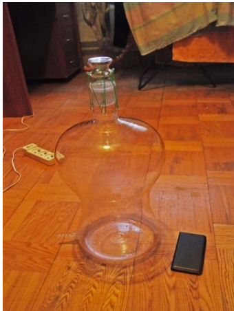
Fig. 13. Borosilicate glass bulb with a neck, hermetically blocked by the plug and the nozzle near the bottom of the bulb
