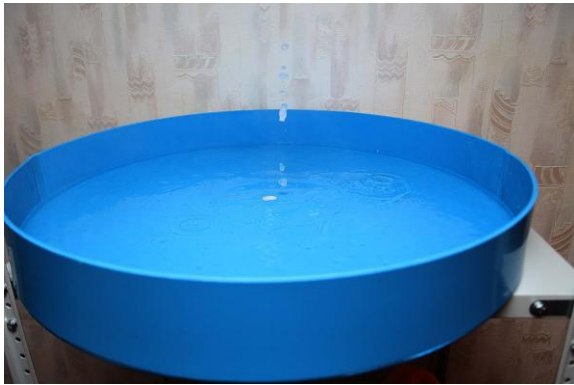
Fig. 16. "Geyser" eruption. Water narrow stream was ejected from the tube together with the vapor
