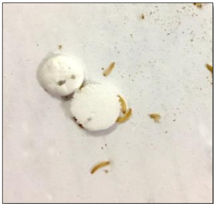
Figure-1: The holes of confused flour beetle, Tribolium confusum inside polystyrene (PS)
