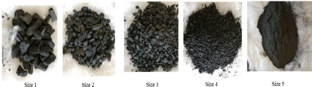
Fig. 1. Sizes of studied biochars as a filter media
