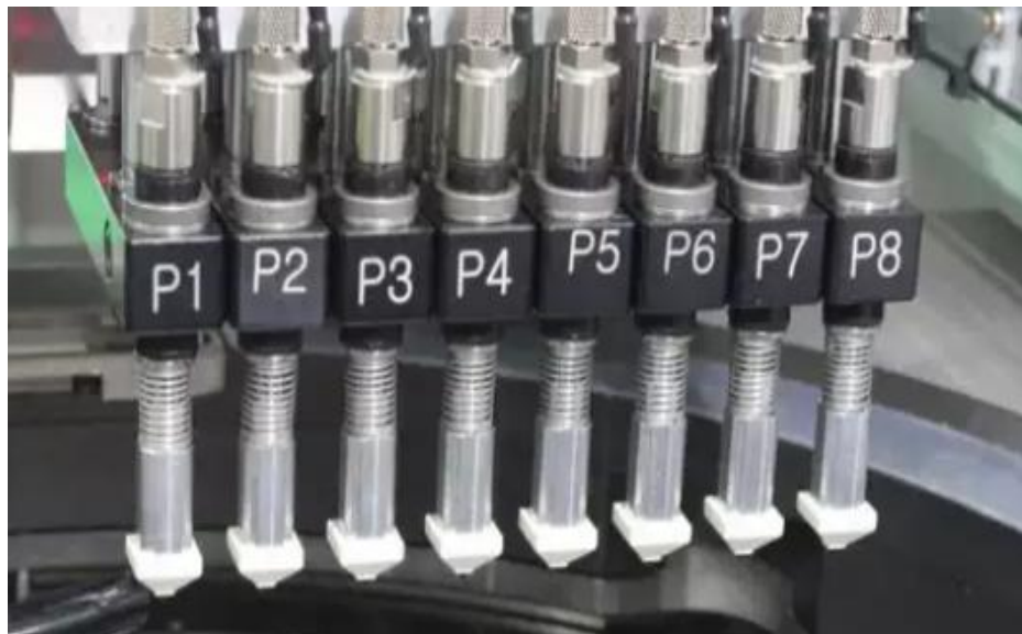
Fig. 1. Z-picker with installed vacuum pads
