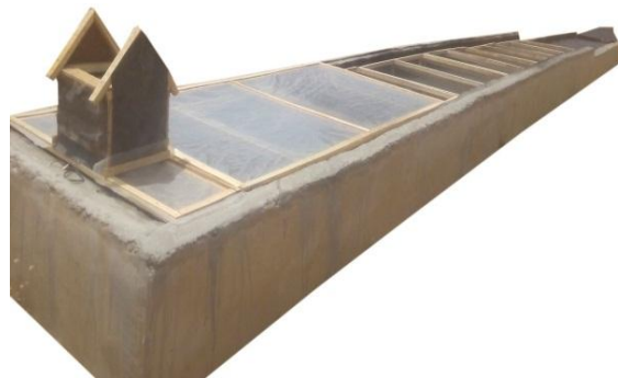
Fig. 1b. Mixed mode on-farm solar dryer
