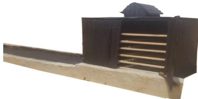
Fig. 1c Indirect mode on-farm solar dryer
