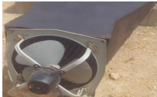
Fig. 1a. Axial Fan Connected to the dryers
