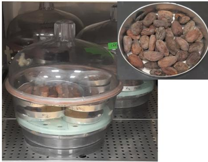
Fig. 1. Experimental cocoa beans storage system in climate chamber
